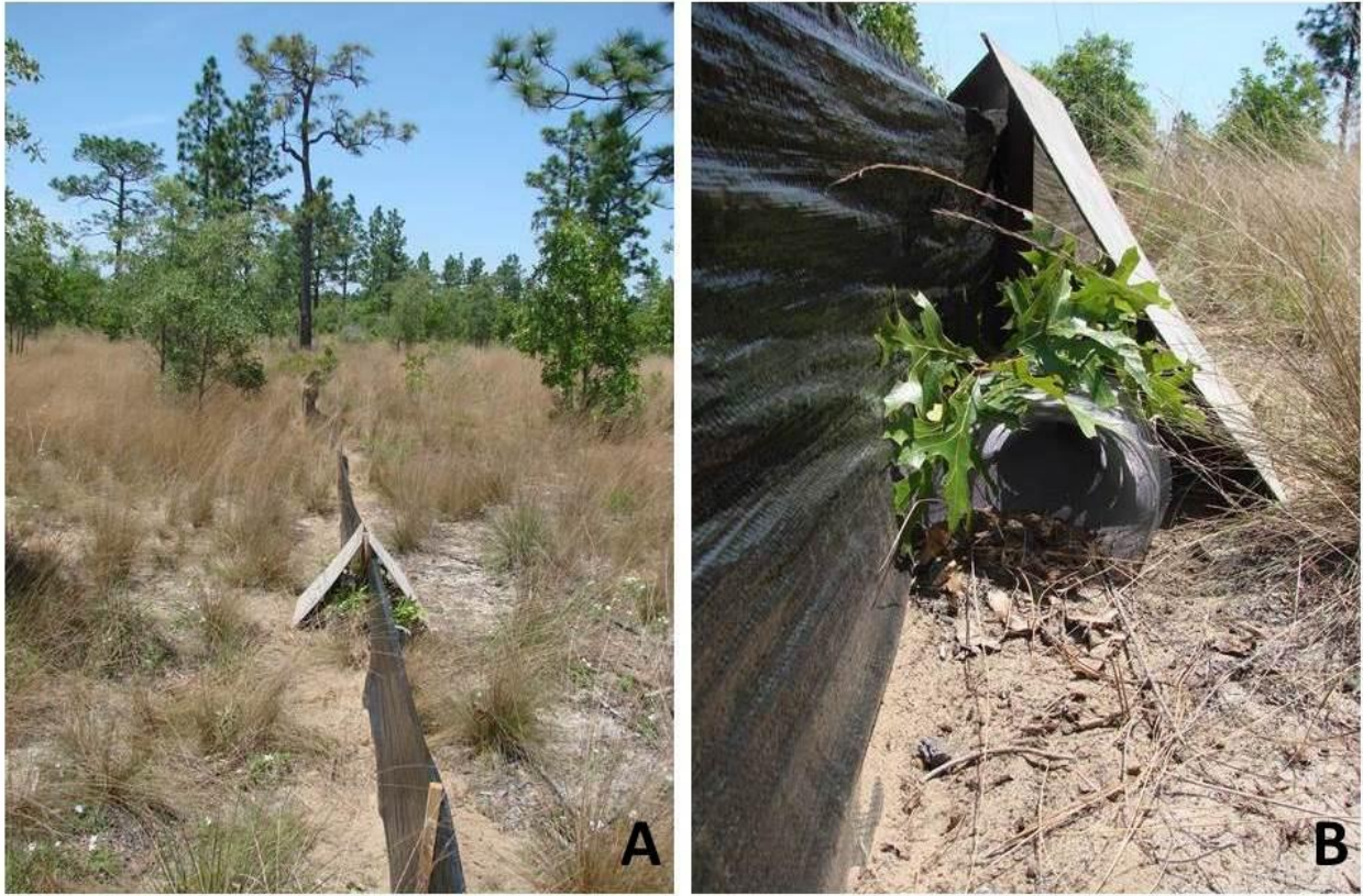
Figure 2. A) A straight-line drift fence for sampling Florida Pine Snakes and Southern Hognose Snakes with B) mesh funnel trap and cover board.
