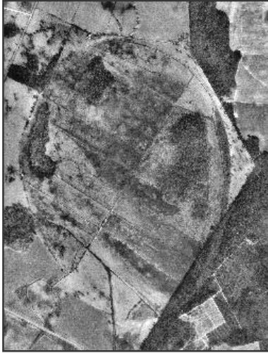
Figure 15. Ditching Intensity = 2 (Intense) Although the outline of this Jenkins County bay can be deciphered, it no longer supports a natural hydrologic regime and no longer supports classic vegetation patterns of bays. There are multiple drainage canals evident in the photograph. The ditches have successfully drained this wetland.
