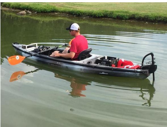
**A converted kayak motorized with a trolling motor. The operator had obtained the required registration and had his life jacket.**
