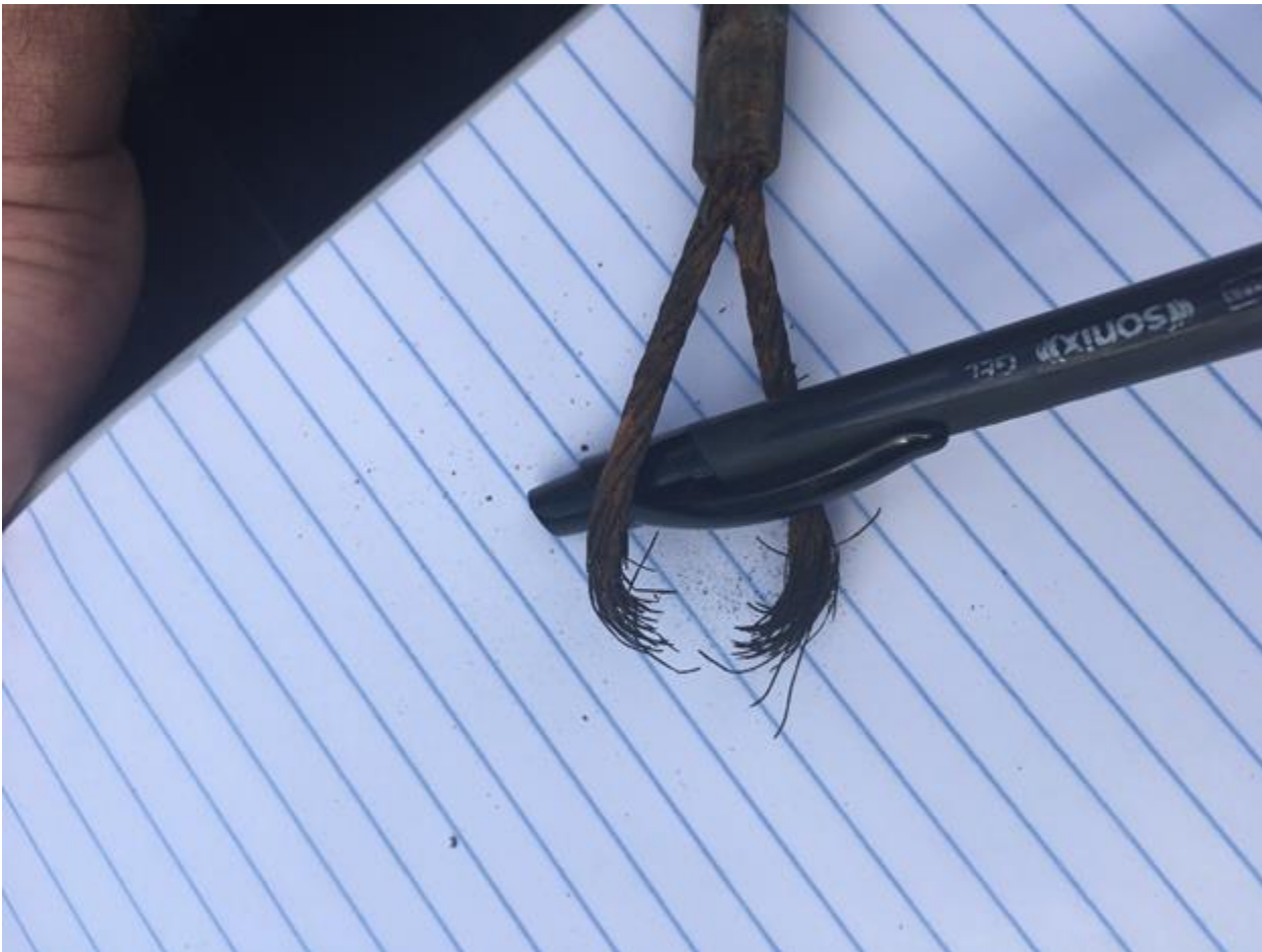
A broken cable was found on a tree stand incident after a hunter fell 10 feet to the ground.
